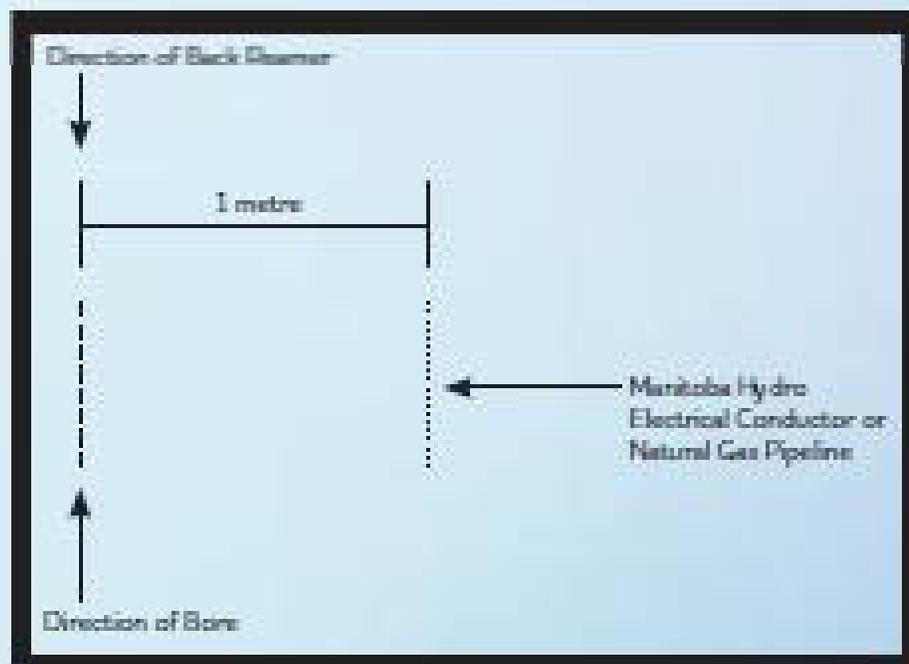
Figure 5: Drilling Parallel to Manitoba Hydro Conductors and Natural Gas Pipelines - Profile View
