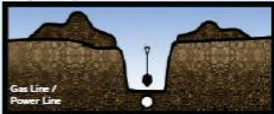
Dig a hole with a shovel directly above the line location until the line is exposed. Take care not to damage the line or coating. Mechanical excavation equipment **MUST NOT** be used to widen or deepen the hole before exposing the line.
