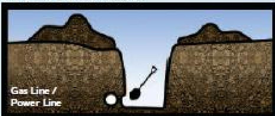
For lines on customer property bringing gas from the main gas pipe to a customer's meter, dig a hole beside the line with a shovel and chip away at the side of the hole to expose the pipe.
