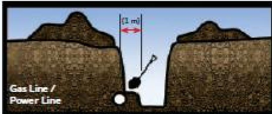
Dig a trench or bell hole 1 metre from the line location, parallel to the line, then hand dig laterally to expose the line.
